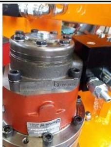
Heavy duty gearmotor equipped with negative brake, overcenter valve and relief valves.
