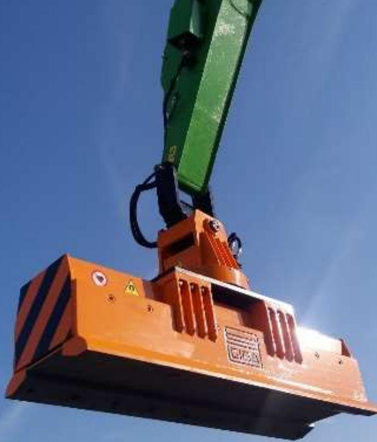
Rotation system with geared slewing bearing and pinion for quick and precise positioning!
